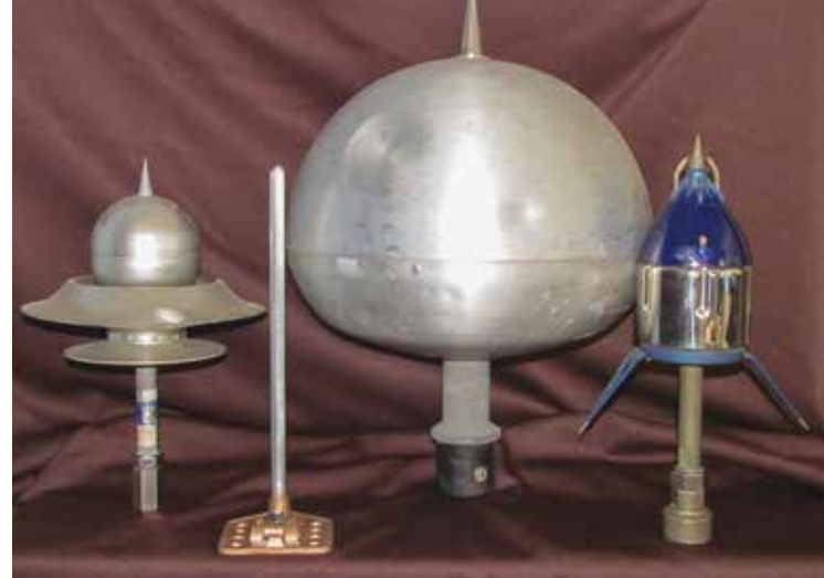
▲ Various types of air terminals are available (left to right): early streamer emission (ESE) device; conventional (conforms to North American standards); a device intended for use with collection volume method calculations; and another ESE device. The non-conventional air terminals were removed from several buildings whose owners opted to replace them with lightning protection systems complying with North American standards.
