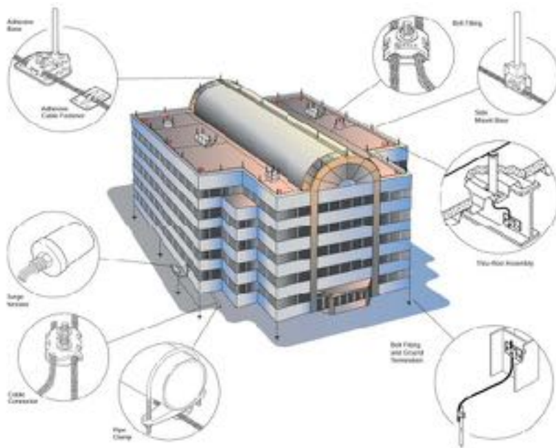
Figure 1: A lightning protection system provides a conductive path that can safely channel lightning into the ground. Air terminals, conductors, ground rods, fittings, and other components must be listed under UL 96—Lightning Protection Components. In most steel-framed buildings, structural members can be used as down conductors between the roof and earth. Surge-protection devices must be installed on all power and signal services penetrating the building envelope. Courtesy: East Coast Lightning Equipment Inc.
