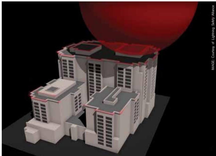
**Figure 1:** A 300-foot-diameter sphere is rolled across a building to model where lightning can strike (shown in red) unless air terminals are provided.
