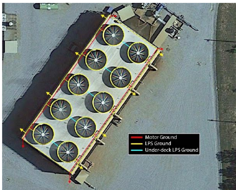
Figure 5: A forensic analysis of lightning-related problems at a power-generating station found several breaches of accepted lightning protection standards. In addition, the motor ground and lightning protection system (LPS) perimeter conductors on this cooling tower (shown in aerial view) run parallel to each other and are separated by only the wall of a nonconducting fiberglass-cable tray. Cooling units that did not have as many lightning-related problems used a different design. Testing identified stray currents that were likely induced currents resulting from the motor ground and LPS perimeter conductors running parallel to each other in close proximity. Courtesy: Scientific Lightning Solutions LLC
